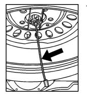
Check under the vehicle to see if the cable end is visible. If the cable is not visible proceed to Step 6.
